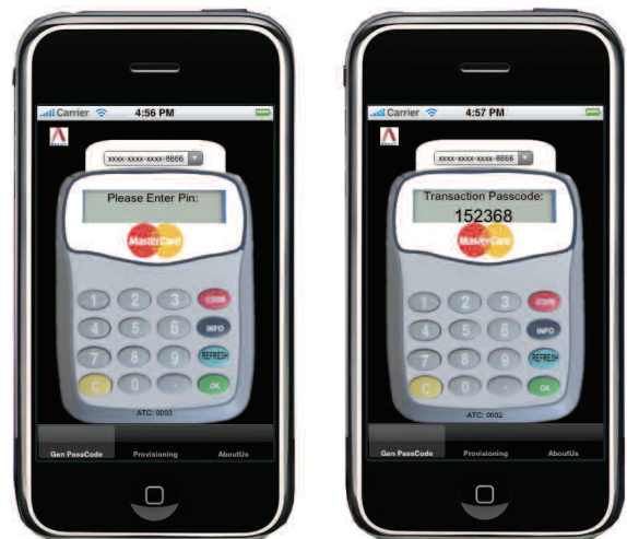
The user can use their mobile phone to automatically generate the one-time-passcode required to gain access to their account or to complete the payment transaction
